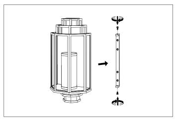
3. Place the lamp over the wall bracket and fix it securely with the screws supplied.
