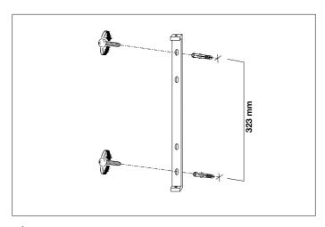
Fix the wall bracket to the wall by using wall mounting plugs and screws suitable to your wall type.
