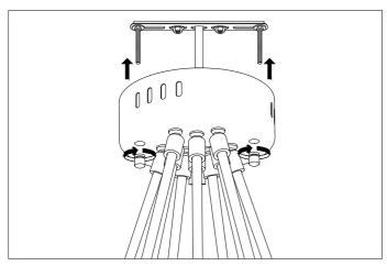
3. Slide the canopy over the ceiling bracket and fix it with the two nuts.
