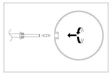
4. Place the G4 lightbulbs and carefully screw on the glass balls, without overtightening them.
