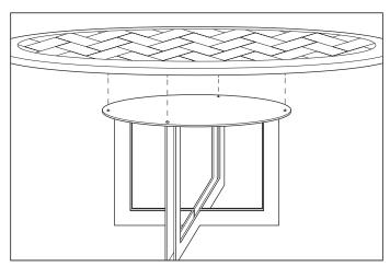
Carefully place the table top on the metal frame and align the holes of the frame with the holes in the table top.
