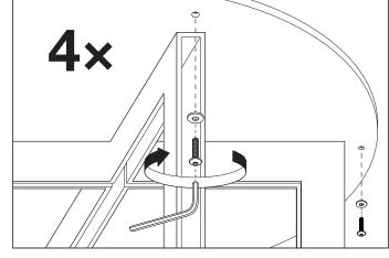
**2.** Fix the table top onto the metal frame by securing the screws with an allen key.
