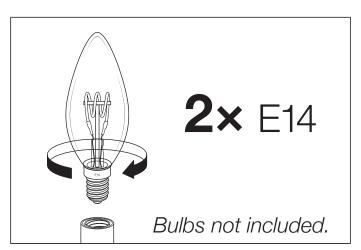
$\bf 5.$  Place the shade and than carefully place the bulbs in the fittings. Do NOT turn the bulbs further than necessary, to prevent damage to the fitting.
