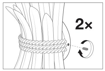
4. Use an allen key to secure the screws on both sides of the lamp.
