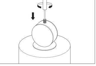
**2.** Determine the desired height of the lamp and connect either one, two or three of the pipes supplied. Thread the wire through the pipes.
