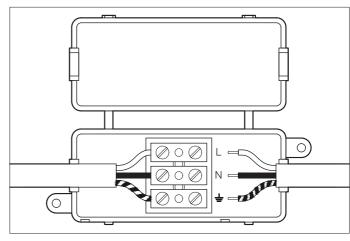
2. Connect the 3 wires according to their colours. Brown is the live wire, blue is the neutral wire,
