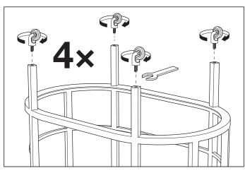
Carefully place the frame of the trolley upside down and fix the wheels to the frame using the spanner (included).
