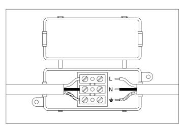
Connect the 3 wires according to their colours. Brown is the live wire, blue is the neutral wire, green/yellow is the earth wire.
