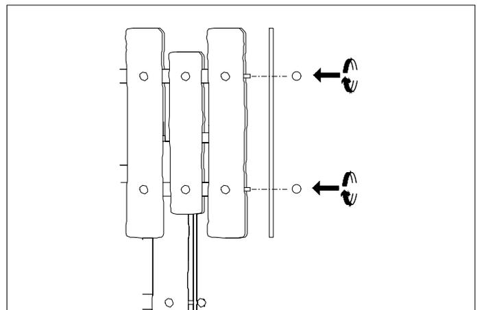
6. Alternately fix the glass to the frame with the screws supplied.
