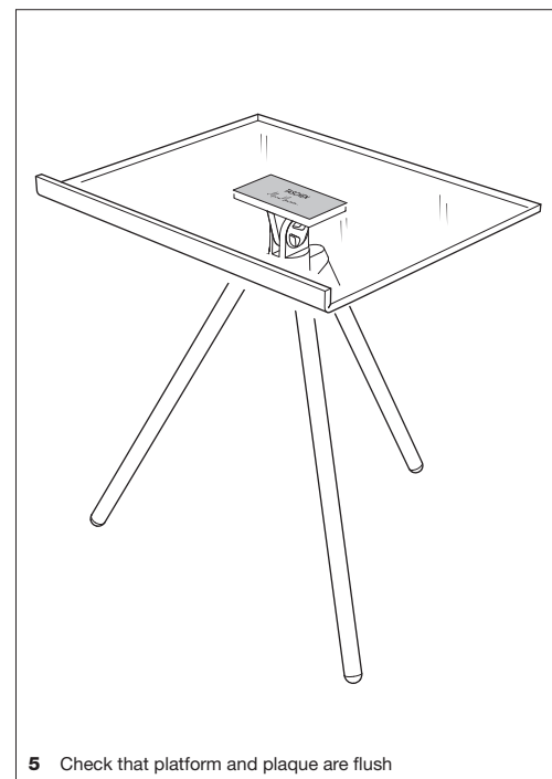
5 Check that platform and plaque are flush
