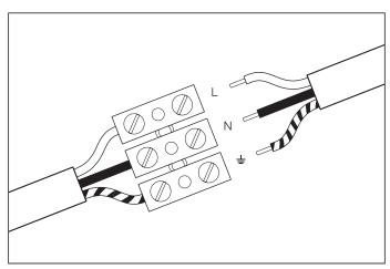
Connect the 3 wires to the LED driver according to their colours. Brown is the live wire, blue is the neutral wire, green/yellow is the earth wire. The LED driver is suitable to be used in combination with a LED dimmer (not included).
