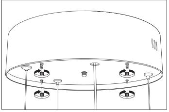
Place the ceiling canopy over the crossbar. Fix the ceiling canopy securely with the nuts.
