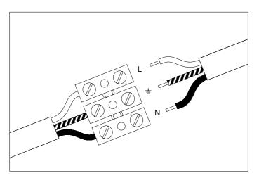
1. Connect the 3 wires according to their colours. Brown is the live wire (L), blue is the neutral wire (N), green/yellow is the earth wire  $(\frac{1}{2})$ .
