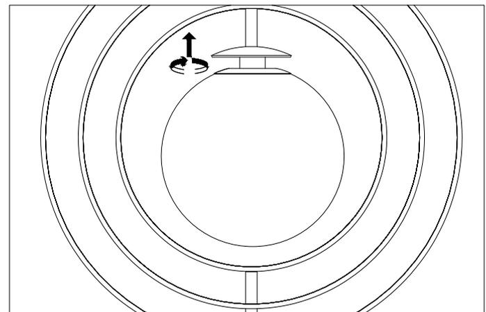
**6.** Place the alabaster glass and adjust the rings to the desired position.
