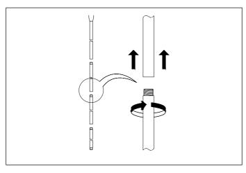
Determine the desired height of the lamp and use either one, two or three of the pipes supplied. Thread the wires through the pipes.
