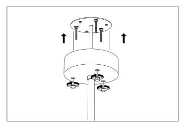
4. Place the ceiling canopy over the ceiling plate and fix it with the three nuts.
