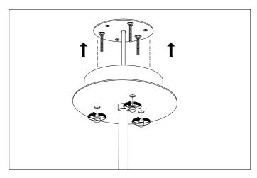
$\textbf{4.} \ \textbf{Place the ceiling canopy over the ceiling plate and fix it securely with the three nuts.}$
