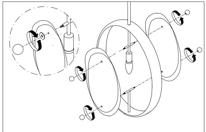
6. Attach the alabaster to the lamp with the screws supplied.
