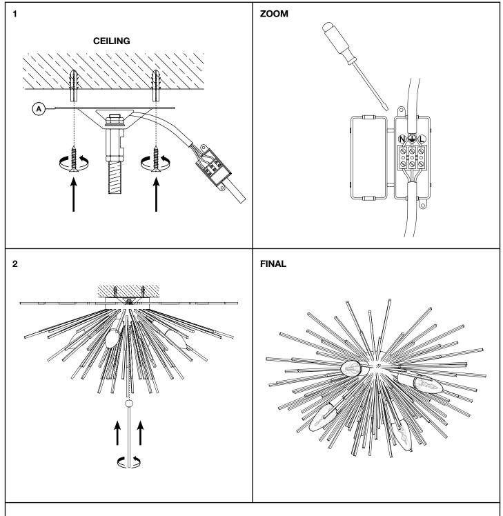
Turn off the electricity supply at the main circuit panel before installing. Do not connect the electricity supply until your luminaire is fully assembled and installed.
