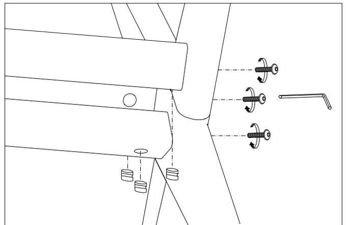
2. Place part C inside the wooden beams. Make sure they are level. If there is resistance while fastening the screws, adjust part C.
