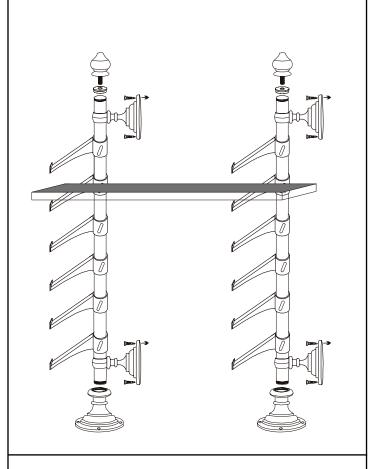
Step 1: Screw the foot (A) to the threaded end of the pole (B).
