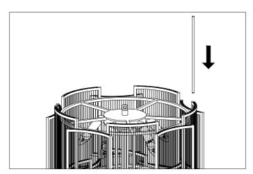
5. Place the glass tubes from the bottom row upwards.
