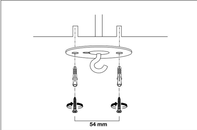
**1.** Fix the ceiling plate to the ceiling by using mounting plugs and screws suitable to your ceiling type. Make sure to lead the wire through the plate.
