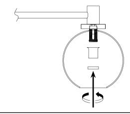
**3** Fix the ceiling plate (A) to the ceiling by using mounting plugs and screws suitable to your ceiling type. Guide the wires through the plate. Place or hold the lamp in an elevated position in such a way that the wires can freely reach the ceiling junction box.
