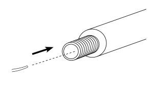
**5** Slide the glass over the lampholder. While holding the glass in place slide the metal sleeve over the lampholder and secure it with the ring.
