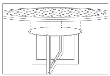
Carefully place the table top on the metal frame and align the holes of the frame with the holes in the table top.
