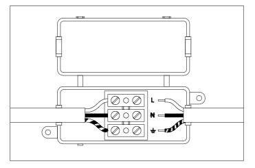
3. Connect the 3 wires according to their colours. Brown is the live wire, blue is neutral wire, green/yellow is the earth wire.
