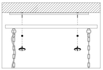
4. Place the canopy over the ceiling plate and fix it with the nuts.
