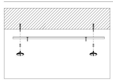
1. Fix the ceiling plate to the ceiling with plugs and screws suitable for your ceiling type.
