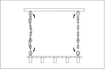
Determine the hanging length of the chandelier. Connect the chain according to the height needed. Thread the wires through the chains and ceiling canopy.
